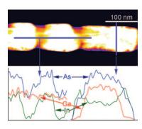
Rings around the wire: Novel hierarchical heterostructures, assembled by radial deposition of InAs on GaAs nanowires with nonplanar side walls, result in the formation of InAs nanorings. The mechanism of formation of such structures, determined by transmission electron microscopy, involves the preferential nucleation of InAs at concave regions of the GaAs surface by capillarity effects.
