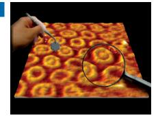
Finding the middle ground: A 1:1 host—guest complex consisting of a hexa-peri-hexabenzocoronene molecule sitting in the middle of the free cavity of a giant  $\pi$ -conjugated carbazole macrocycle has been obtained (see STM image). The complex has been prepared by physisorption of a monolayer of macrocycles followed by gas-phase deposition of graphene molecules by pulsed laser deposition.
