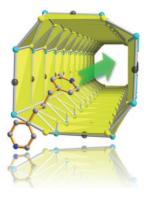
Glowing with pride: An activator-free gallium oxalatophosphite is a new class of color conversion phosphors for NUV and blue light-emitting diodes. It is synthesized by using an organic template and an environmentally friendly eutectic solvent in a reaction that shows efficient atom economy. The resulting material has a tubular structure (see picture) and intriguing luminescence properties.
